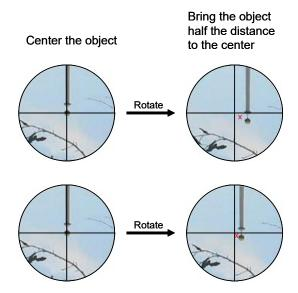
9. After few times, the object will stay in center when the mount is flipped from right to left.
