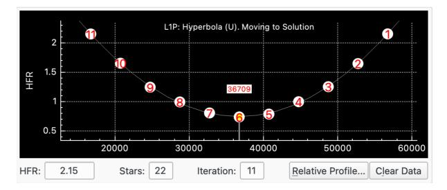
6. Up until this point, the Linear 1 Pass algorithm is very similar to the Linear algorithm. The next step in Linear 1 Pass is different though. The focuser is moved directly to the focus minimum in a backlash independent way (see the Backlash section). The R2 value of the curve fit is calculated, and the final V-Curve displayed. The title summarises details of the solution including the R2 value.
